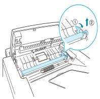
4 Wipe the roller surface with a soft cloth dampened with water.
